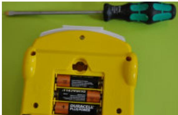
Batteries can be replaced in the back of the robot. Please use a screwdriver to open the battery compartments. The top compartment contains 3 AA batteries. The smaller compartment contains one C2032 battery.
